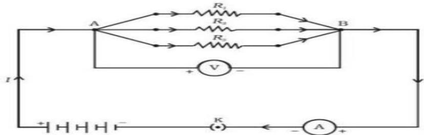
$$V/R = V/R_1 + V/R_2 + V/R_3$$
