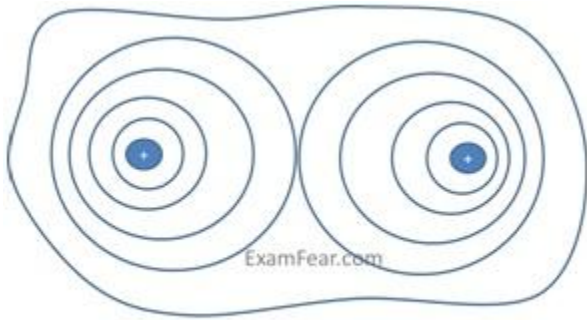
Equipotential surface for two identical charges
